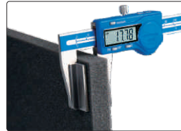
Measure thickness of rubber
